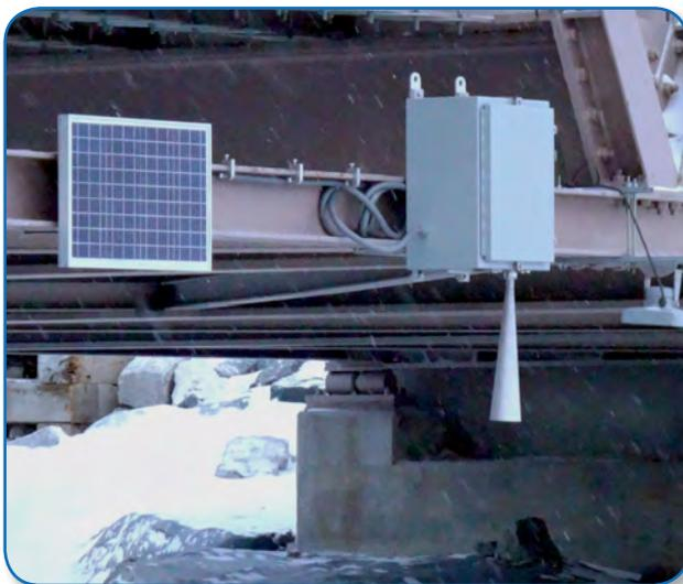
The station will take 15 minute measurements for water level, air temperature, and relative humidity. Once an hour this data will be transmitted via the Iridium Satellite network to the SutronWIN database. With custom log-in information, approved end users can view all data in table and graph formats as well as download the data.
