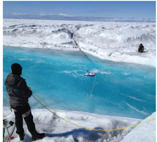
*UCLA graduate student Lincoln Pitcher and University of Wyoming graduate student Brandon Overstreet measuring discharge in a supraglacial ice river on top of the Greenland Ice Sheet, immediately following record melting in July of 2012.*
