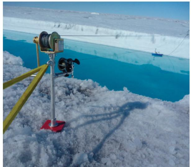
*One side of the cableway was secured to the stream bank using ice screws. The cable was tensioned using a hand crank and the RiverSurveyor was attached to the cable*
