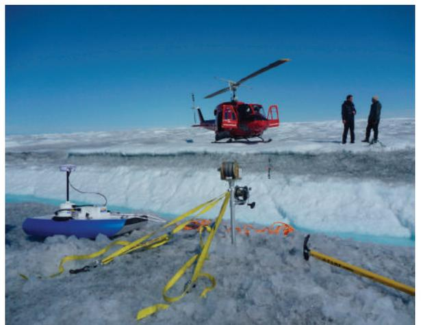
*A second operator was flown across the stream by helicopter and a second anchor system was installed.*
