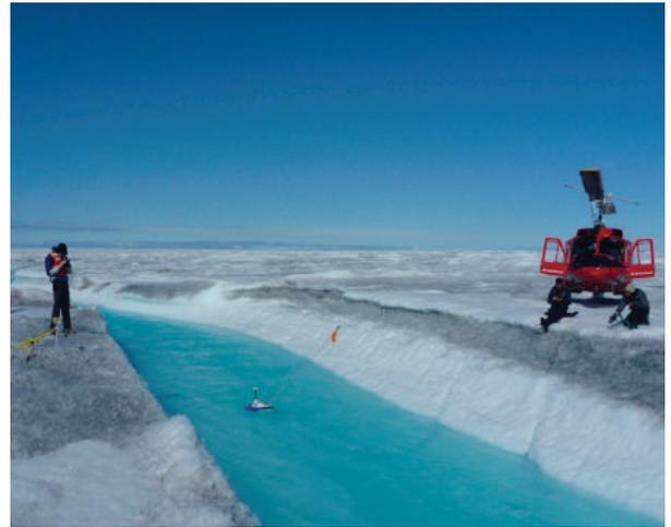
*The RiverSurveyor was operated via mobile phone while being slowly pulled across the stream.*
